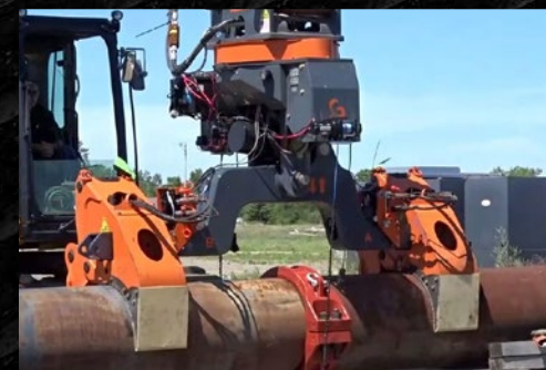
U-Beam Design for Mechanical Pipe Joining
